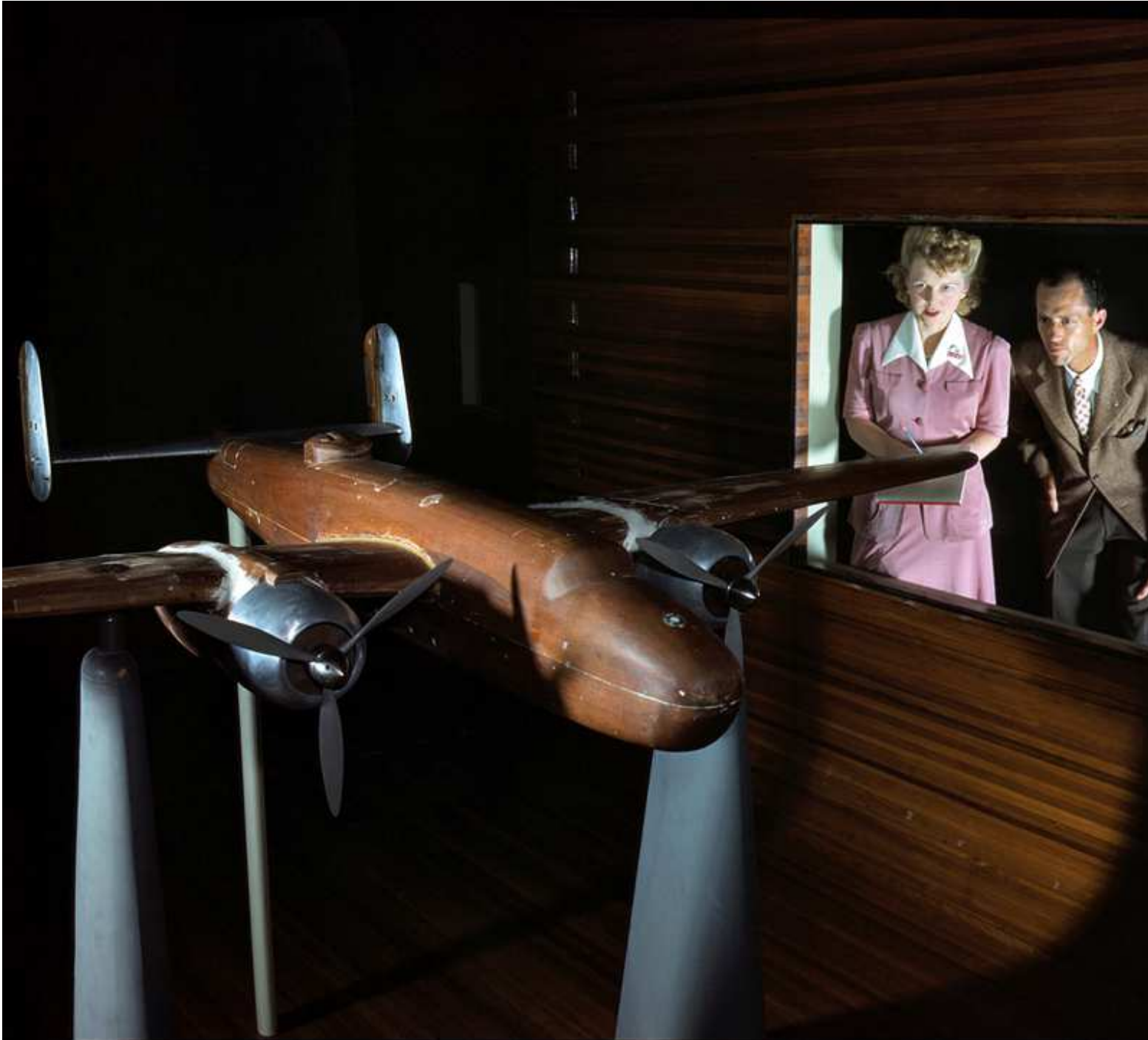
October 1942. Experimental staff at the North American Aviation plant in Ingle- wood, Calif. , observing wind tunnel tests on a model of the B-25 ("Billy Mitchell") bomber. 4x5 Kodachrome transparency by Alfred Palmer.
