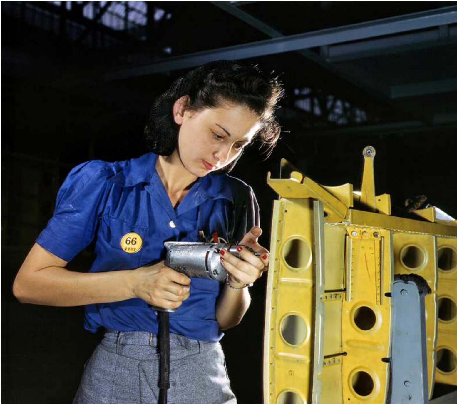
February 1943. Working on the horizontal stabilizer of a "Vengeance" dive bomber at the Consolidated-Vultee plant in Nashville . 4x5 Kodachrome transparency by Alfred Palmer for the Office of War Information.
