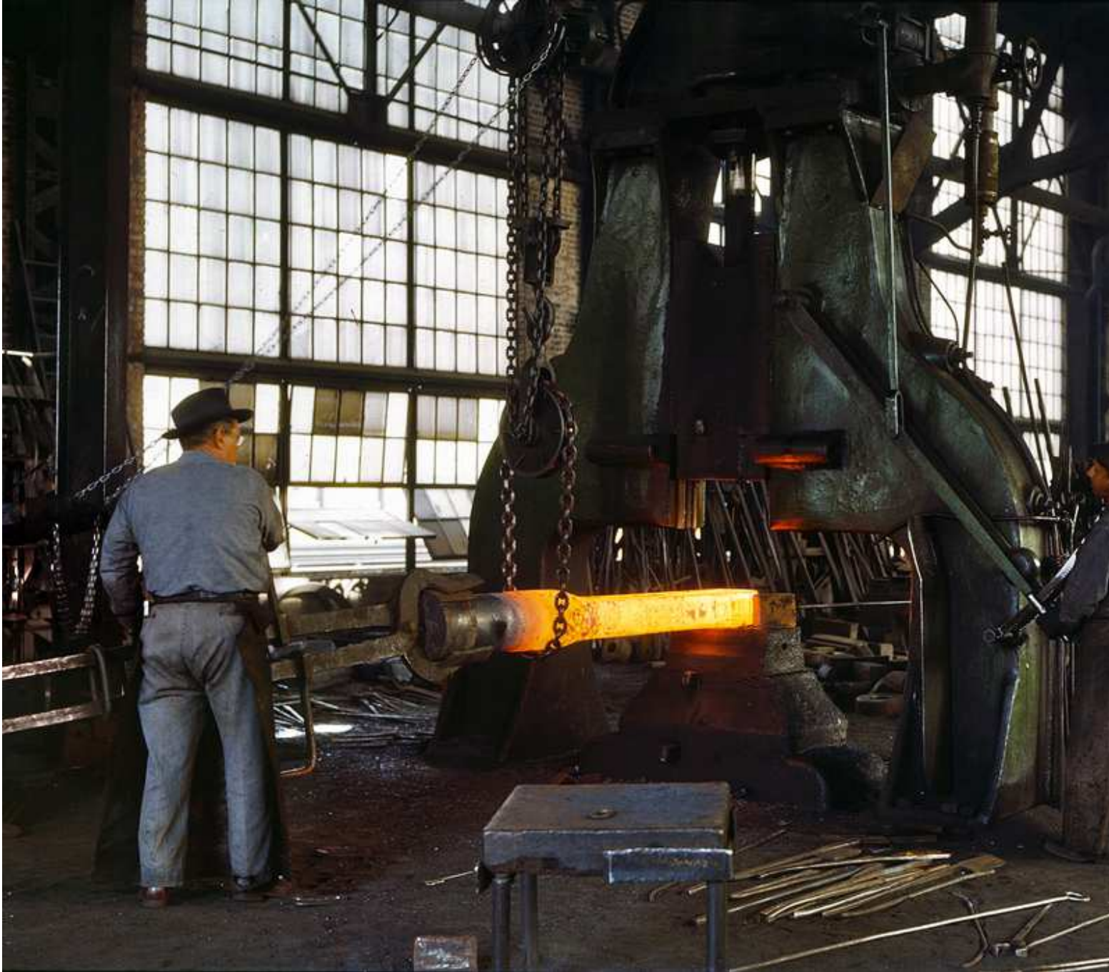
March 1943. "Santa Fe R.R. shops, Albuquerque . Hammering out a drawbar on the steam drop hammer in the blacksmith shop." 4x5 Kodachrome transparency by Jack Delano for the Office of War Information.
