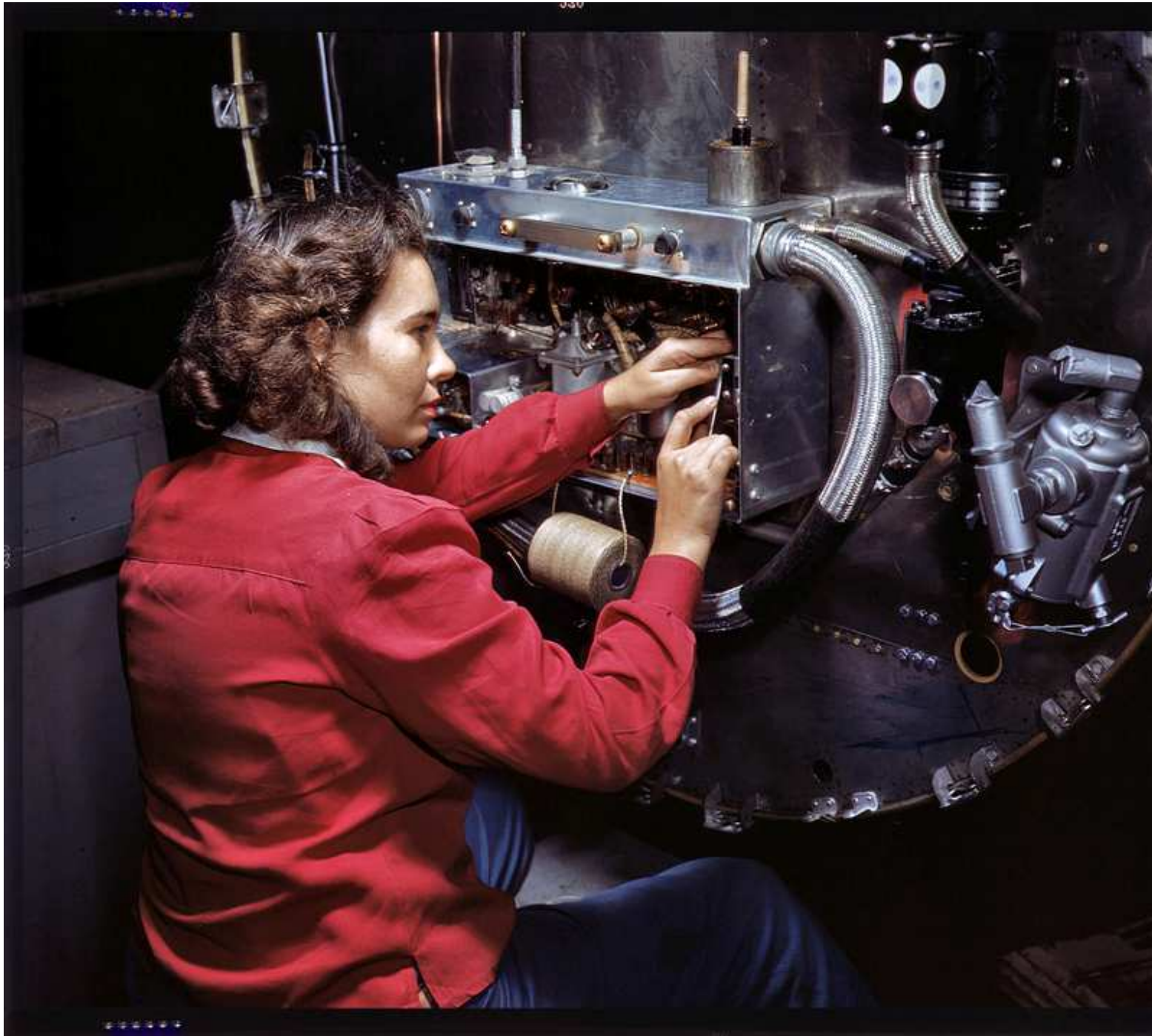
October 1942. Assembling switchboxes on the firewalls of B-25 bombers at North American Aviation's Inglewood , California , factory. 4x5 Kodachrome transparency by Alfred Palmer, Office of War Information.
