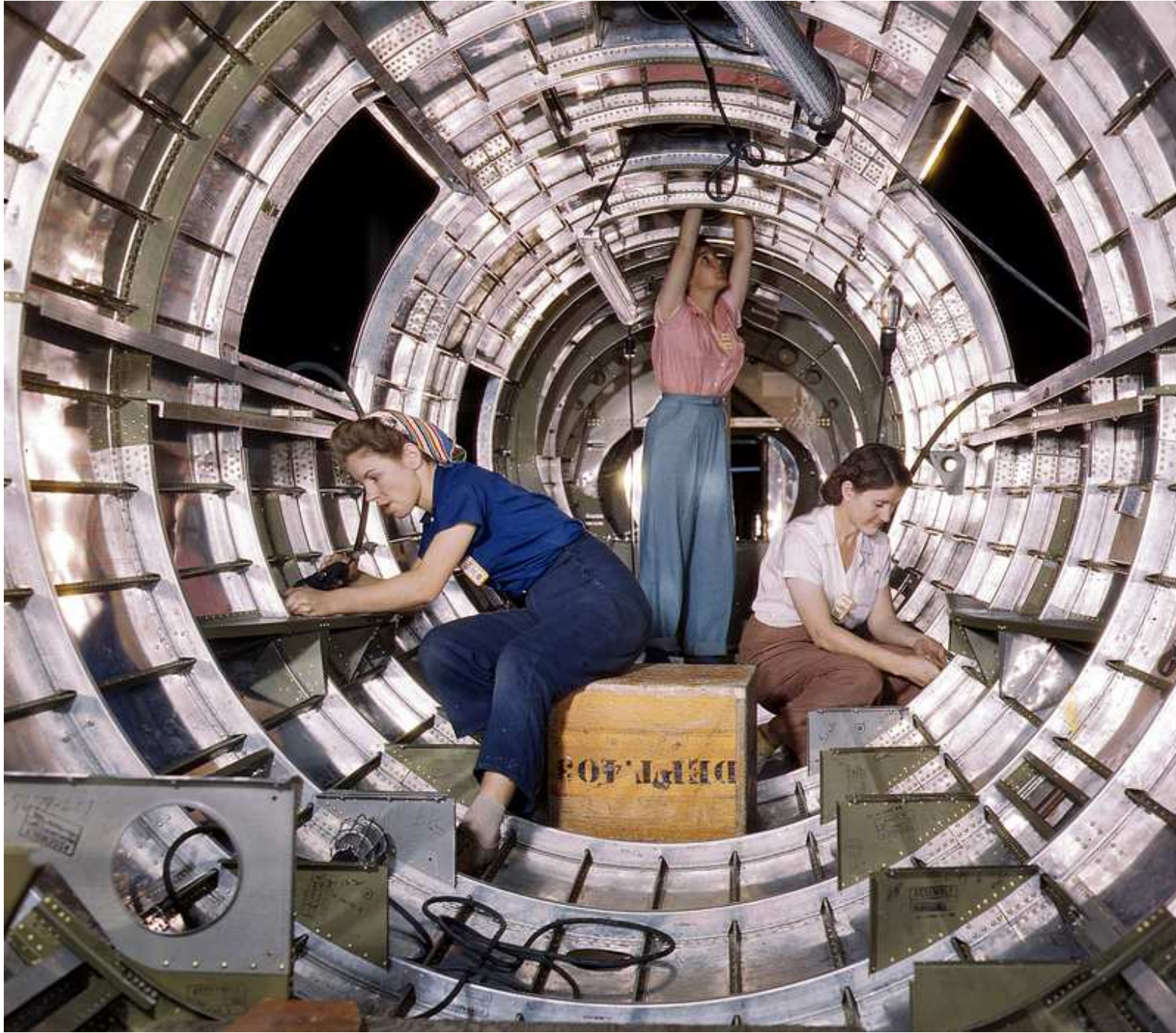
October 1942. Workers installing fixtures and assemblies in the tail section of a B-17F bomber at the Douglas Aircraft Company plant in Long Beach , California . 4x5 Kodachrome transparency by Alfred Palmer.
